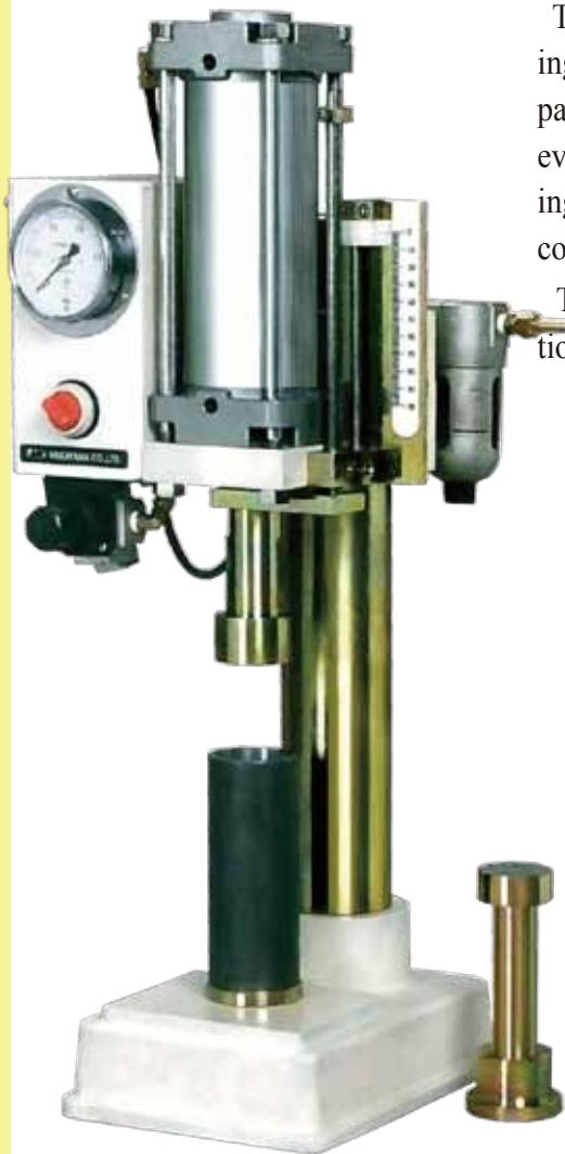
This is for measuring compactability of molding sand, consisting of an air pressure type tester and a sample holder. Compactability test is a quantitative replacement of a qualitative evaluation of molding sand by the feel of a palm when squeezing sand. Amount of moisture and clay in sand as well as oolitic content and degree of mulling can be evaluated by this test.
